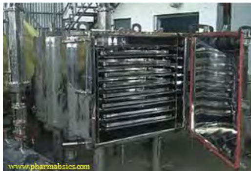
Gambar 38. Contoh pengering vakum ( vacuum dryer )
