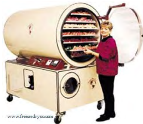
Gambar 40. Contoh pengering beku ( freeze dryer )
