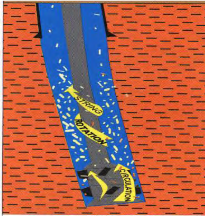
Gambar ; Pipa terjepit (Pipe Stuck)
