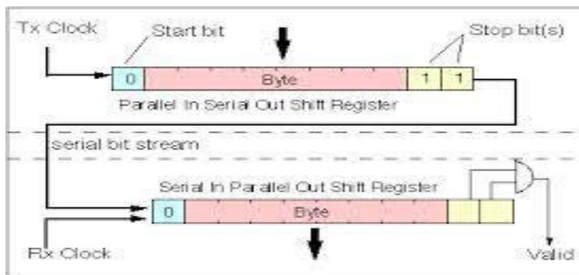
**Gambar 21** asynchronous transmission
