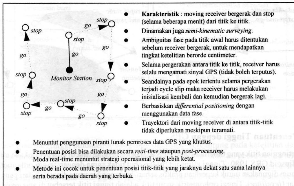
Gambar 4.17. Metode penentuan posisi stop and go
