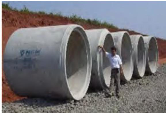
Gambar 1.25. Pipa beton
