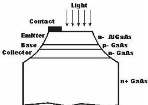
Gambar 5.4.2 struktur Hetero mesa- phototransistor
