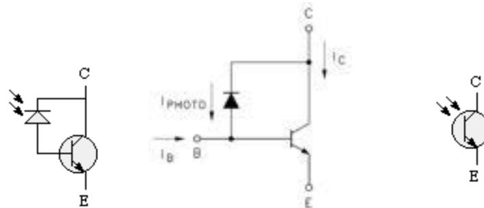
Gambar 5.4.3. simbol Phototransistor
