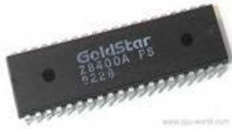
Gambar 1.7. IC Intel 8080 dan Goldstar Z8400A 4MHz/40-pin plastic DIP
