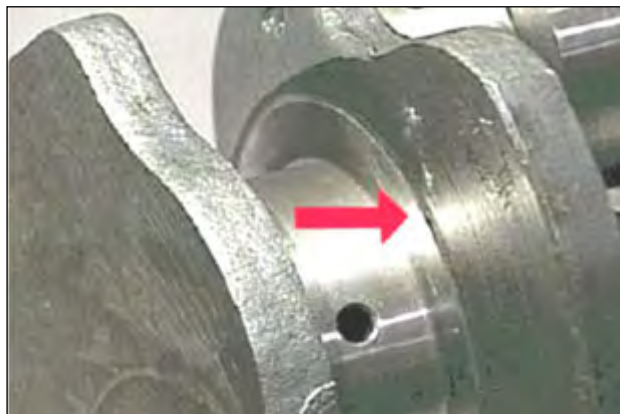
Gambar 3.104. Permukaan Thrust Bearing
