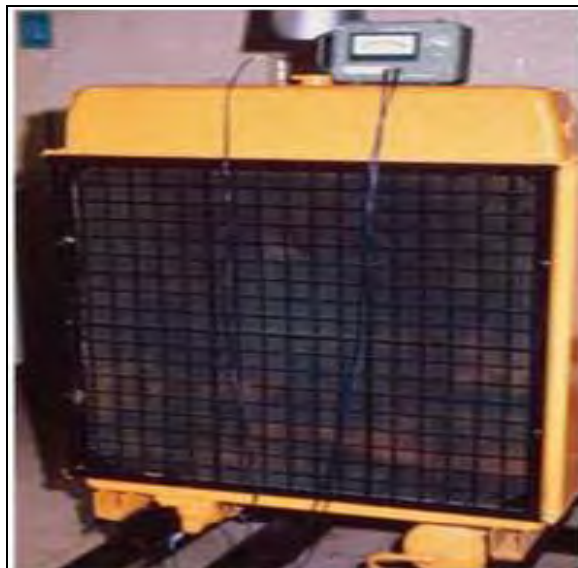
Gambar 10.102 Hambatan aliran coolant
