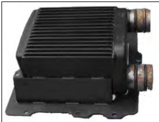
Gambar 32 Jacket water aftercooler
