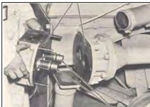
Gambar 10.117 Periksa kondisi thermostat housing
