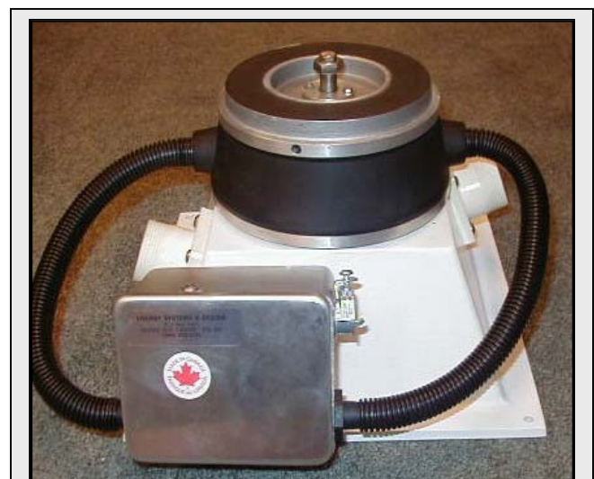
The Stream Engine with the Turgo runner housed in the white casing, the permanent magnet alternator on top and the controller in the foreground (silver box)
