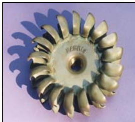
Close-up of the Harris Pelton Turbine runner
