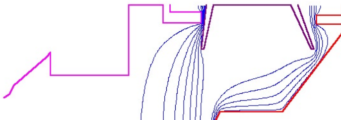
Figure 13: Equipotential Lines in a three stage collector. The potentials are determined by collector geometry and collector voltages.
