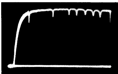
Fig. 913. Display obtained in check of generator flatness. A marker box provides absorption markers.
