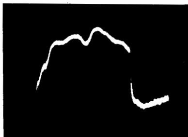
Fig. 1010 (left). Display of 60-cycle wave, low-capacitance pickup. Fig. 1011 (right). Observation of details by trace expansion and off-centering.
