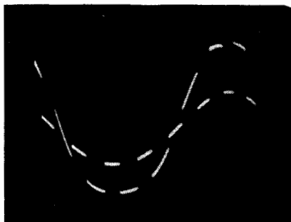
Fig. 301. By means of an electronic switch the spot successively writes two traces or parts thereof.
