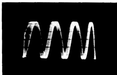
Fig. 1023 (left). Hum in the X amplifier. The whole trace is shifted back and forth. Fig. 1024 (right). Time-base hum. While one end of the trace remains stationary, the other end is swept back and forth.
