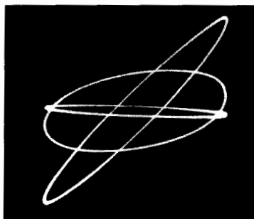
Fig. 521. Phasing ellipses obtained with the same values of R as in Fig. 518.
