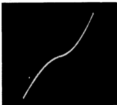
Fig. 642. Characteristic of a non-linear thyrite resistor (varistor).
