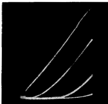
Fig. 619 (left). I_p/E_p characteristics of a 12AX7 for bias voltages from 0 (top) to -3 volts (bottom). Fig. 620 (right). Reducing the sweep voltage results in incomplete curves.
