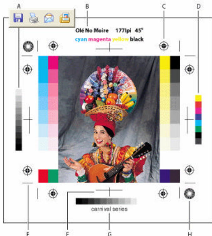
Page marks A. Gradient tint bar B. Label C. Registration marks D. Progressive color bar E. Corner crop mark F. Center crop mark G. Caption H. Star target
